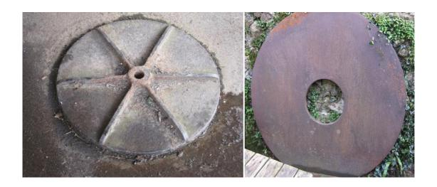
The wheelwright would place a newly made cartwheel on the plate, threaded over a vertical bar with the hub resting in a hole in the ground. The wheel was held in place by a cover fitted over the bar. The blacksmith would measure the wheel, cut his iron to size, and
